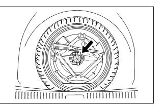
4. Turn the wing nut to remove the retainer that holds the wrench and jack.
